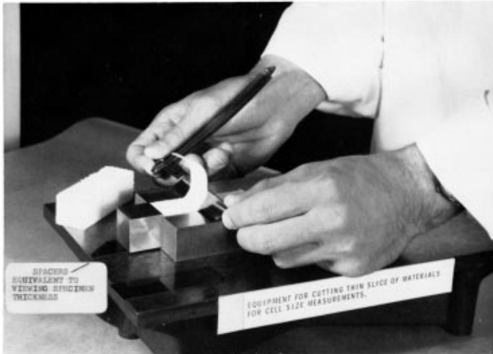
FIG. 1 Razor Blade Cell Size Specimen Slicer
